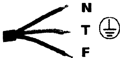
Figure 4: Power and grounding cables
